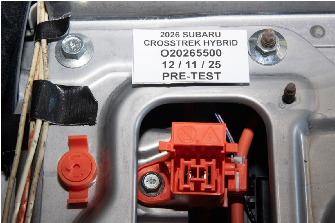
FIGURE 305-06. Manual High Voltage Service Disconnect Removed
