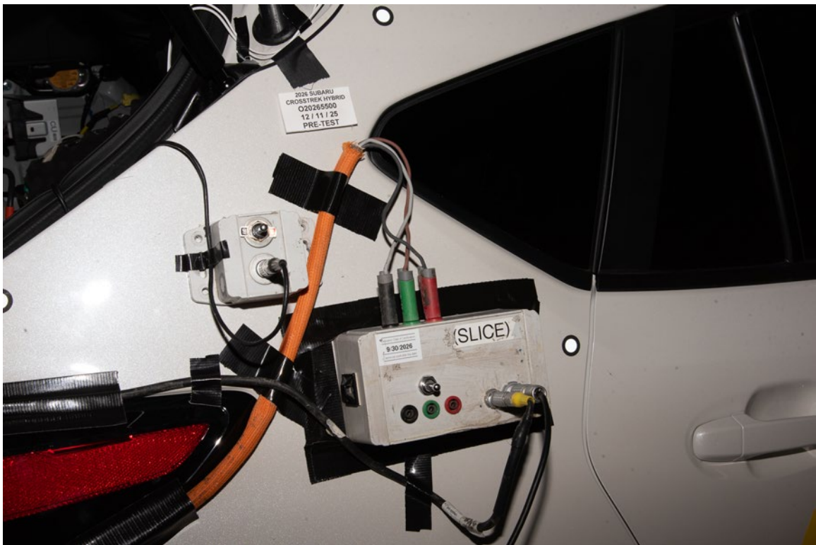
FIGURE 305-013. Pre-Impact View of Installed Test Interface Port
