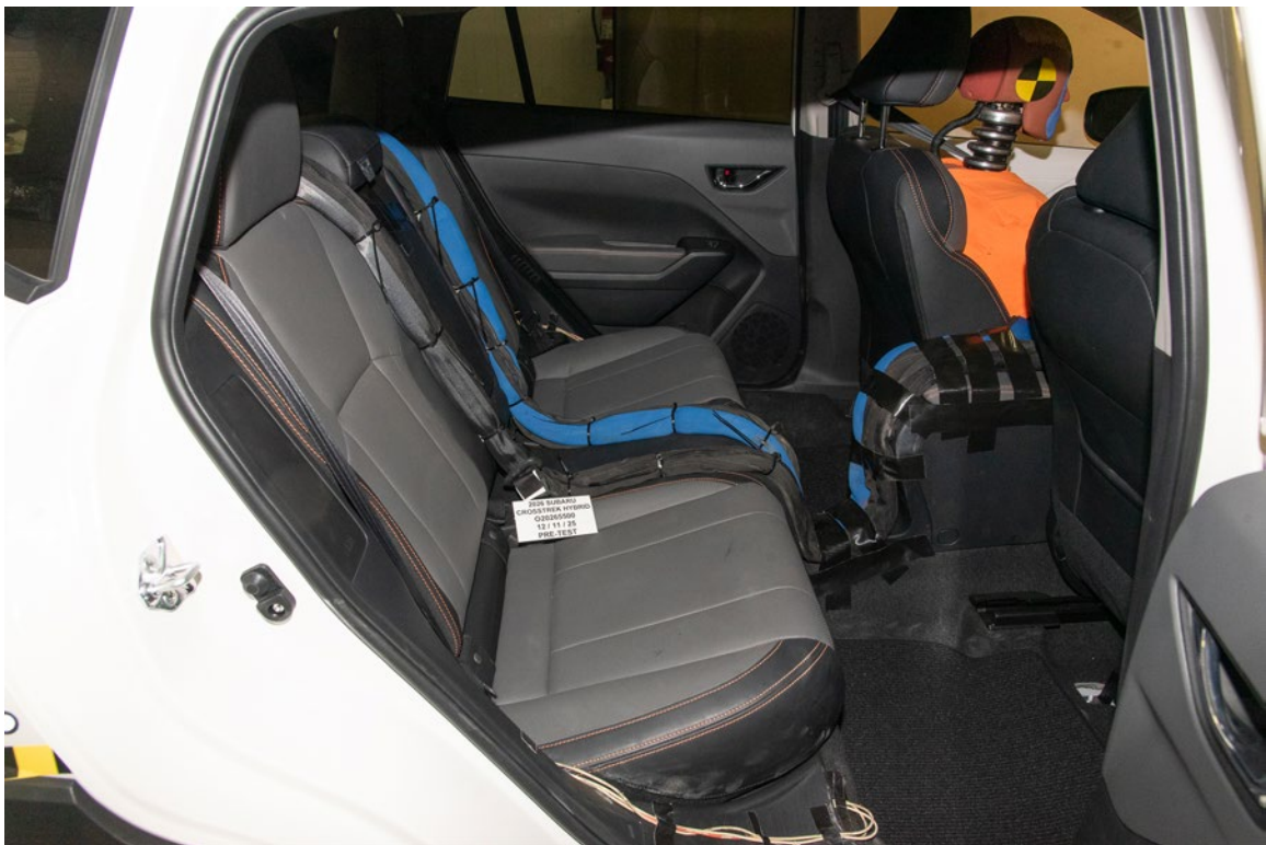
FIGURE 28. Pre-Test Dummy Cable Routing
