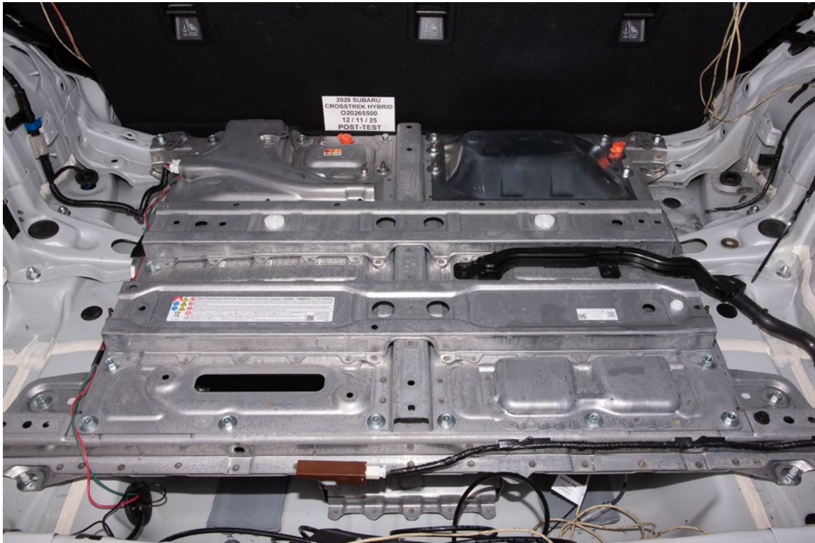
FIGURE 305-08. Post-Impact Rear View of Propulsion Battery
